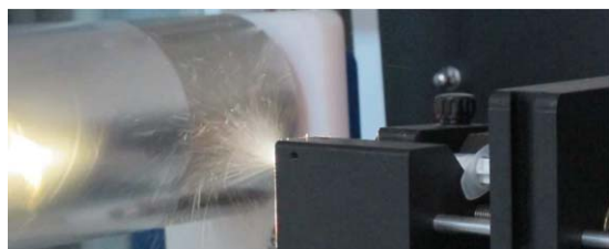
Figure 9. Photo picture of electrospinning of MWCNT/HBPE/THF solution under the conditions of Run 1A in Table IV. [Color figure can be viewed in the online issue, which is available at wileyonlinelibrary.com .]
